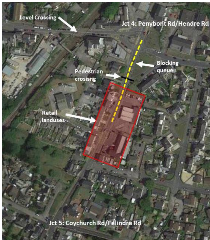
Figure 2: Queuing on Coychurch Road Impeding Hendre Road Junction
